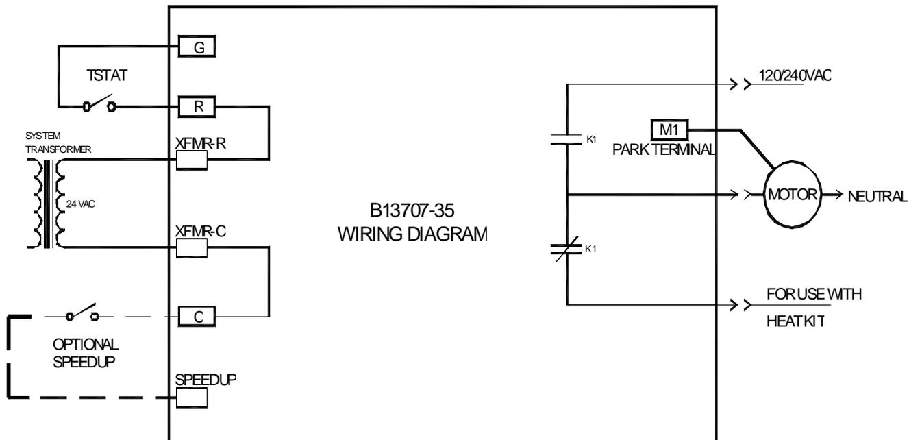
The Electronic Blower Time Delay Relay provides power to the blower motor with a delay of 7 seconds after 24VAC is applied to "G". After 24VAC is removed from "G", the blower motor output is de-energized after a delay of 65 seconds.
