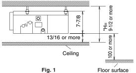
Select the \*H dimension such that a downward slope of at least 1/100 is ensured as indicated in "7. DRAIN PIPING WORK".
