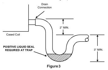
The depth of a running trap should be either 1" or a depth that permits unrestricted condensate drainage without excessive air discharge.
