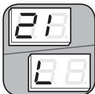
Active Protection – Code 21L – Open low-pressure control
