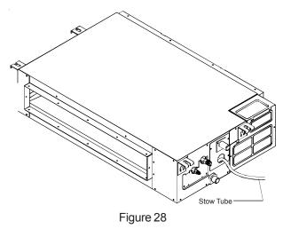
3. Restore power to the unit and operate the air conditioner under the COOLING mode. While listening to the sound of the drain pump, check to see if the water is discharge properly.
